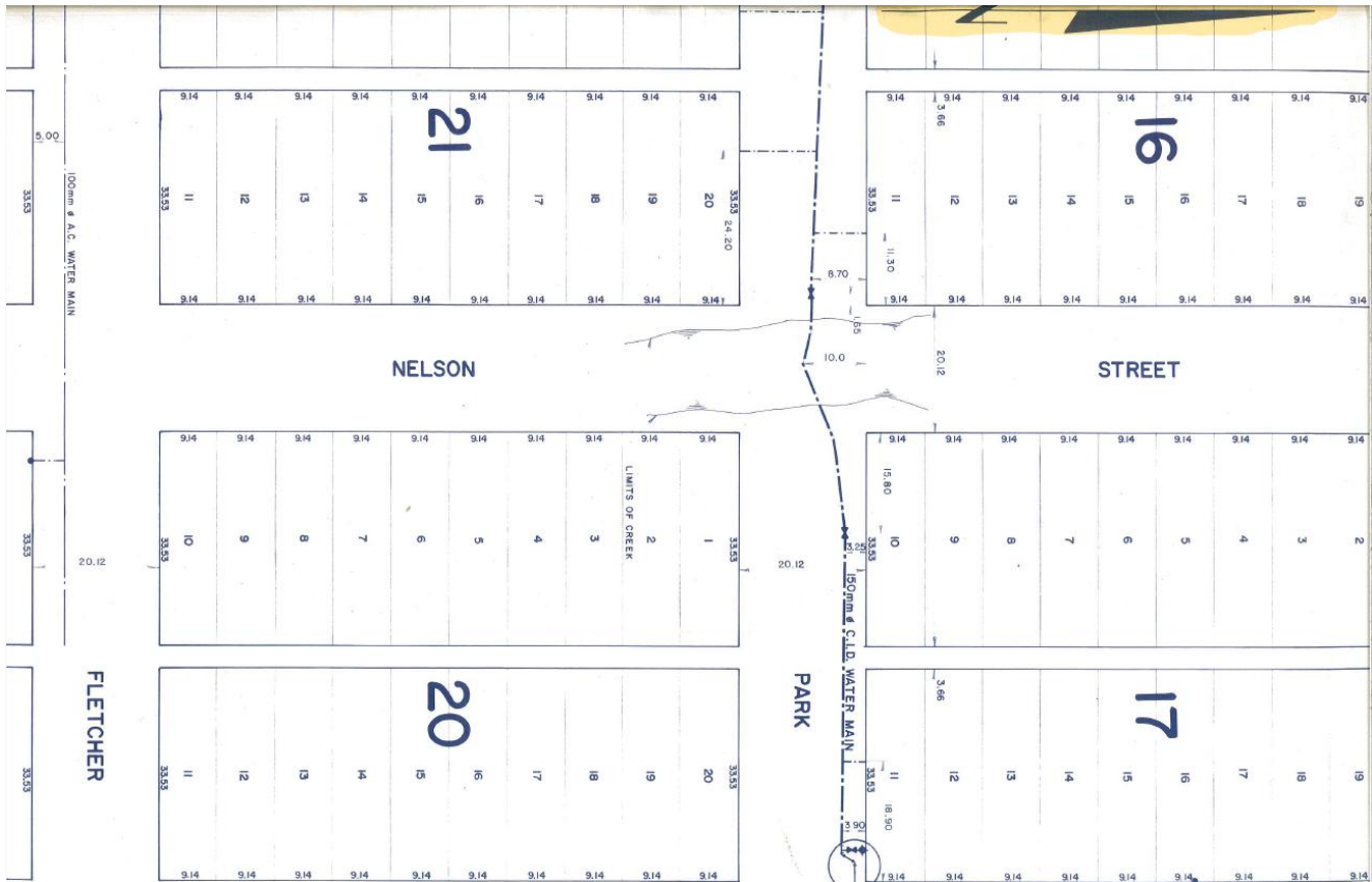
FIGURE 1 – PARK AVENUE WATER MAIN CROSSING:
