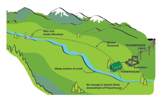
Run of river hydropower is a type of waterpower generation that has been used throughout the world for over 100 years.
